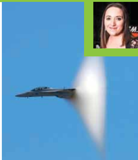
Condensation shock associated with local supersonic flow.
